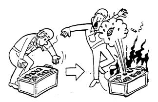
DON'T smoke near the battery Never use an open flame as a light anywhere on or around the battery. Battery gas is highly flammable. Sulfuric acid is destructive. If it comes in contact with your skin, wash it off at once with water.
