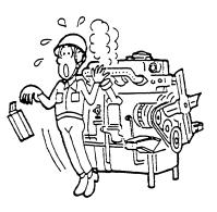
DON'T touch hot engine parts such as exhaust manifolds.
