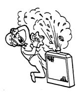
DON'T remove radiator filler cap immediately after shutting down engine.
